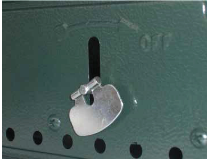
Figure 8 Auxiliary Burner Control
