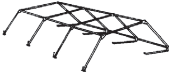
Figure 8 Erect One Side
