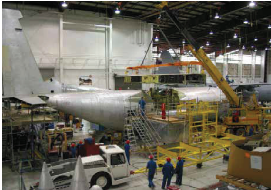
Figure A-1 Rebuilding a C-130 Centre Wing
