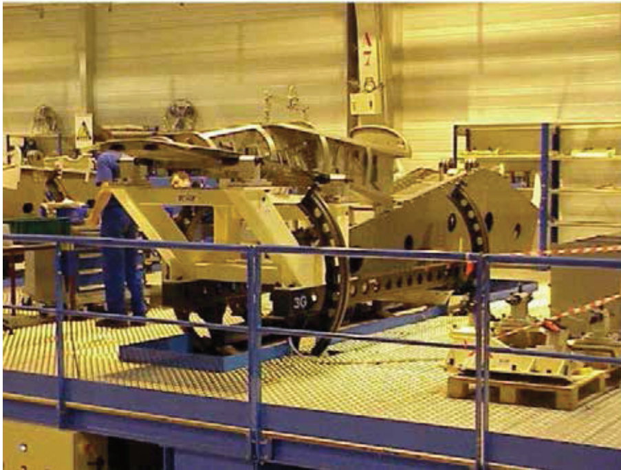
Figure B-1 Building a Pylon
