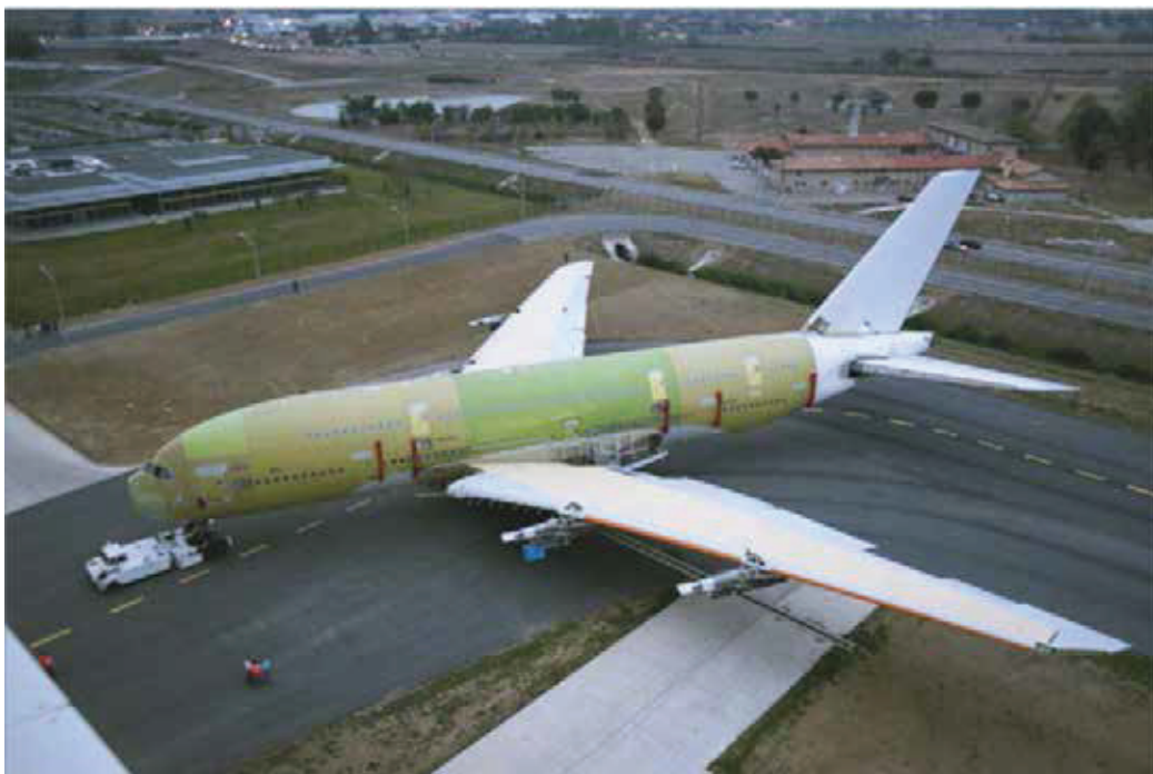
Figure B-4 Empty Pylons
