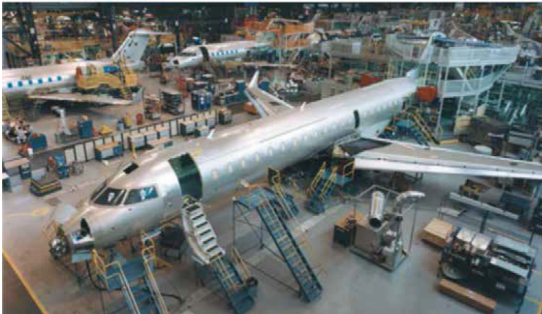
Figure A-10 Bombardier CRJ700 Assembly Line
