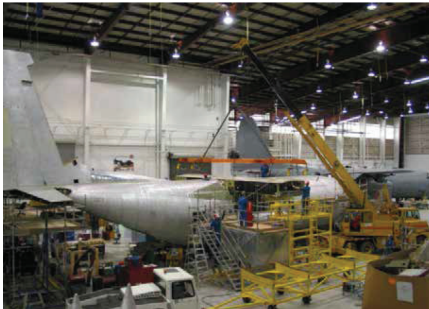
Figure A-2 Placing a C-130 Centre Wing
