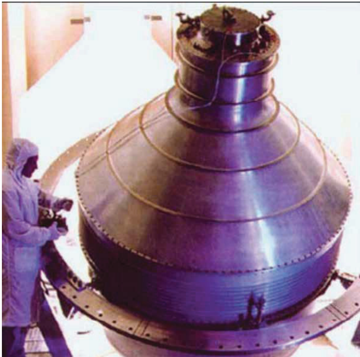
Figure A-2 Gravity Probe B Dewar
