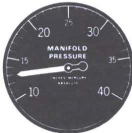
Figure A-4 Manifold Pressure Gauge
