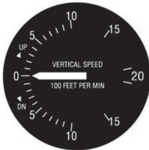
Figure 17B-3 Vertical Speed Indicator Parts
