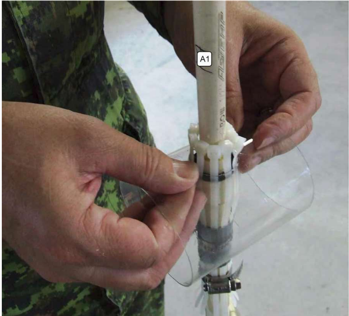
Figure 28-A Sliding the Spring over the Cable Ties
