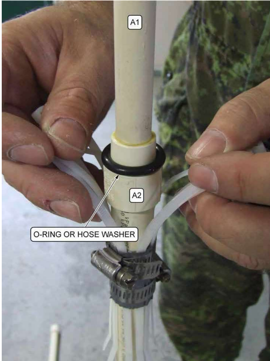
Figure 23-A Position of the O-Ring or Hose Washer on A2
