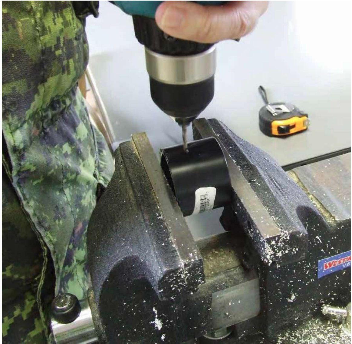
Figure 26-A Drilling 1/8-inch Holes in the ABS Coupler
