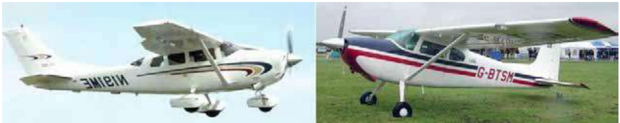
Figure 3 Nose Gear v. Tail Gear
